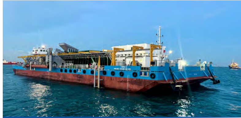
Subsea rock installation barge performing sea trial
