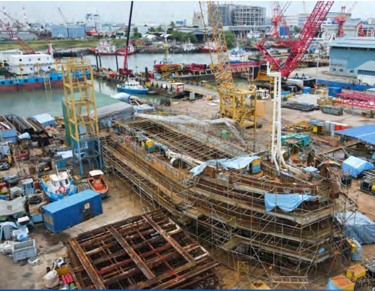
New build – 680m 3 Self-Propelled Split Hopper Barge
