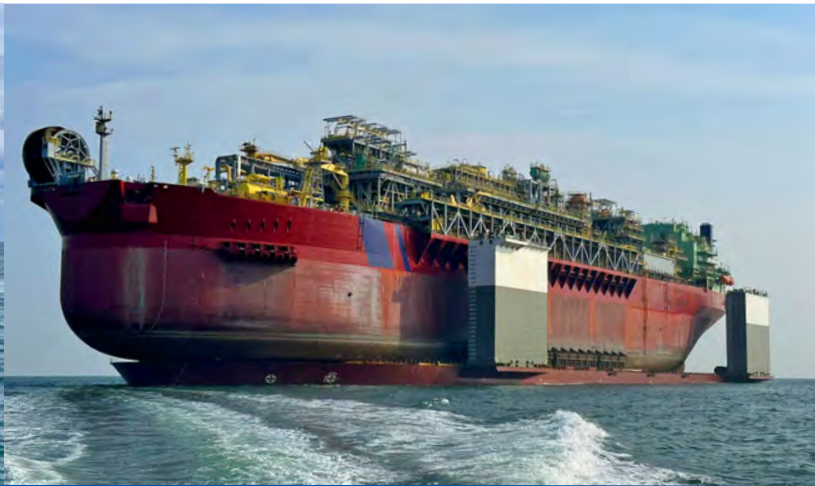
Loading operations for Floating Production Unit OPPORTUNITY
